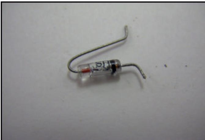
**Fig. 13 – Diode D1 prepared for soldering.**
