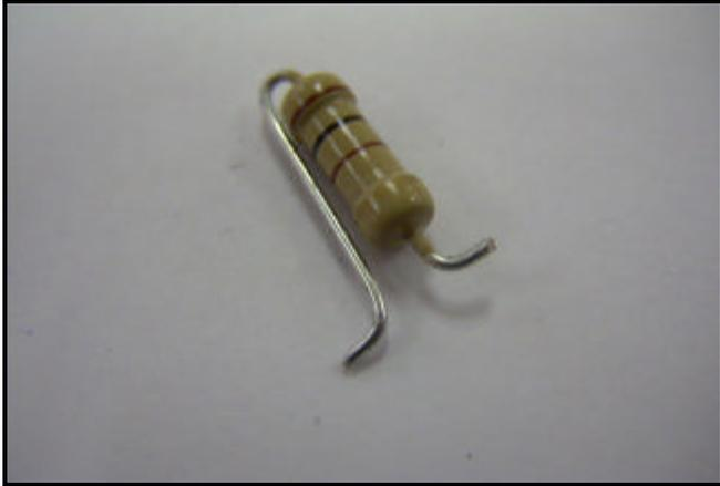
**Fig. 7 – 100 ohm Resistor ready to mount**
