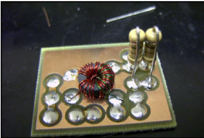
**Fig. 8 – Resistors R2 & R2A Mounted.**
