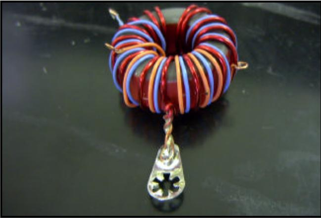
**Fig. 29 – The large toroid prepared for mounting.**
