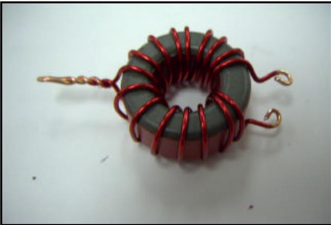
**Fig. 26 - L1 wound on the red core.**
