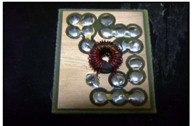
Fig. 6 – Toroid Mounted on Board
