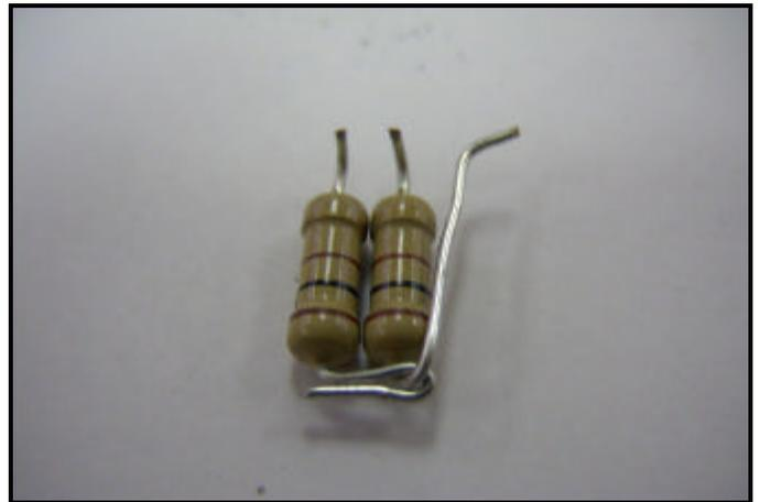
**Fig. 9, Resistors R3 & R3A ready to solder.**
