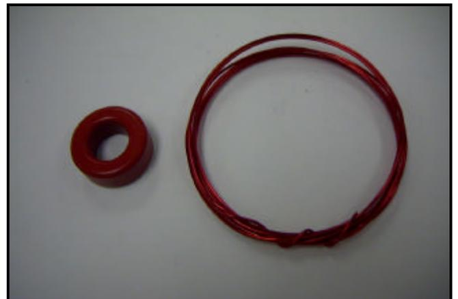
**Fig. 24 – Red Toroid and Heavy Wire.**
