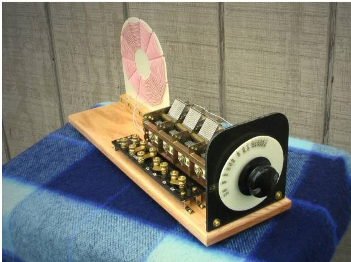
There are 4 uses I have found for this tuner. (This is why I call it a *multi-use* tuner.) The first use is a front end for my medium wave dx crystal or tube regenerative radios. Second is using the 4 gang capacitor with a loop antenna as a high performance crystal radio. Third is a long wave tuner and finally a signal booster for a nearby radio. Please look at the circuit below as I describe the different uses.
