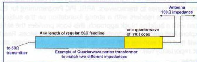
**FACT 6.** Parallel coaxes can be utilised to match a number of situations with a little creativity when the formula comes out to non-standard transmission line. This diagram shows how to make up a 35Ω quarter wave matching section, required to match the 25Ω of two paralleled 50Ω antennas to a 50Ω feedline.
