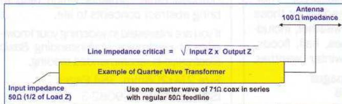
**FACT 5.** If we needed to match a 100Ω antenna to a 50Ω coax, a quarter wave piece of 70Ω coax in series with the regular line would do the job. Just insert the quarter wave piece before the antenna and you have a good match. (Note: a quarter wave transformer only works at one frequency. It is not a broadband device.) For frequencies
