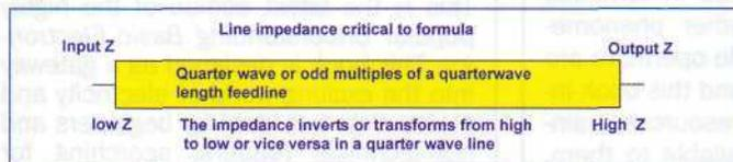
**FACT 4.** To utilise this concept to match two unequal impedances, multiply the two impedances on each end and take the square root. This becomes the necessary impedance of the quarter wave transformer. You will have to obtain (cut) a quarter wave piece of transmission line made to this impedance. If it's an odd number (not 50 or 75Ω) it can be creatively obtained by paralleling lines or other means.
